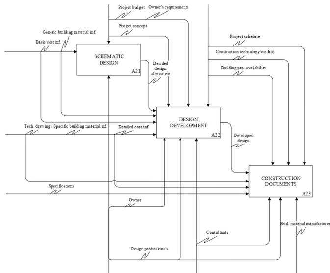
Figure 4. IDEF-0 diagram representing design phase building production selection process.
