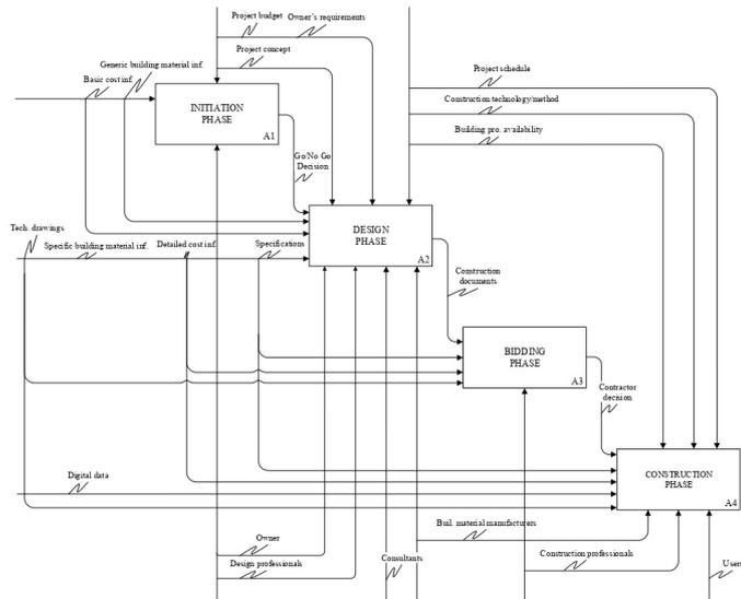
Figure 3. IDEF-0 diagram representing building production selection process.
