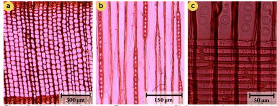
**Figure 7.** Abies bornmuelleriana. a- Transverse section: Distinct growth ring boundaries, b-Tangential section: Uniseriate rays, average ray height is 15 to 30 cells. c- Radial section: Homocellular rays, tangential walls of rays distinct nodular chains. cross-field pits taxodioid, usually uniseriate, sometimes biseriate pits in radial tracheid walls. The scale bar for a= 300  $\mu$ m, for b= 150  $\mu$ m and for c= 50  $\mu$ m.
