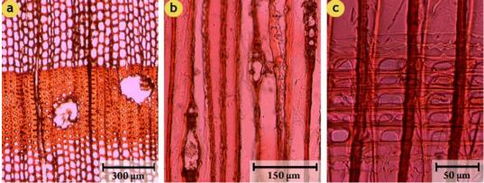
**Figure 9.** Pinus slyvestris. a- Transverse section: Distinct growth ring boundaries, large resin canals with thin-walled epithelial cells. b- Tangential section: Rays with resin canals. c- Radial section: Heterocellular rays, ray traheids with dentated walls, cross-fields from parenchyma cells to tracheids with one (rarely two) large fenestriform pits. Tracheid pits almost uniseriate. The scale bar for A= 300  $\mu$ m, for B= 150  $\mu$ m and for C= 50  $\mu$ m.
