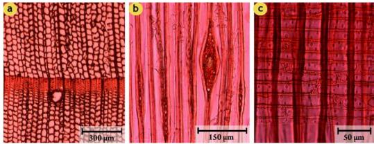
**Figure 8.** Picea orientalis. a- Transverse section: Distinct growth ring boundaries, surrounded by thick-walled epithelial cells. b- Tangential section: Rays with resin canals. c- Radial section: Heterocellular uniseriate rays, ray traheids with smooth walls, cross-field pits piceoid, longitudinal tracheids generally with uniseriate, rarely biseriate pits. The scale bar for A= 300  $\mu$ m, for B= 150  $\mu$ m and for C= 50  $\mu$ m.
