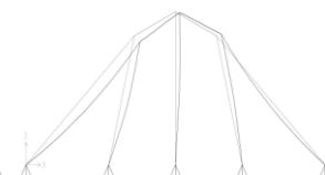
Figure 20: Deformation diagram of the hung system tent
