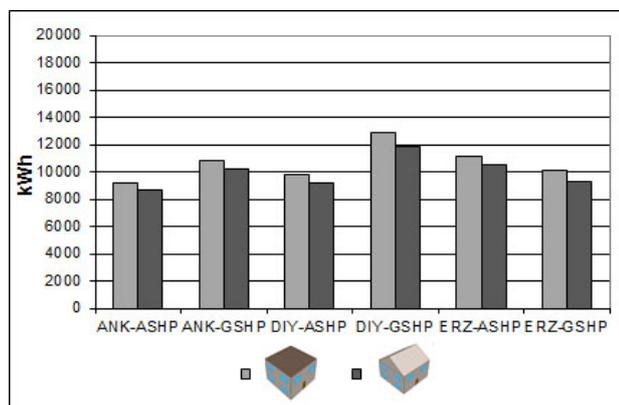
**Figure 4.** The comparison of annual energy consumption of flat and pitched roof when ASHP and GSHP systems are used in Ankara, Diyarbakir, Erzurum for square building form.
