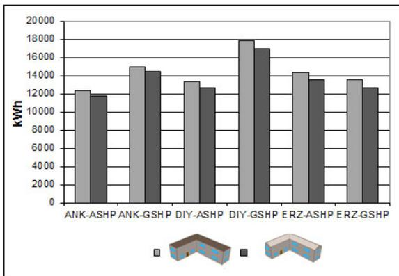
**Figure 6.** The comparison of annual energy consumption of flat and pitched roof when ASHP and GSHP systems are used in Ankara, Diyarbakir, Erzurum for L-shaped building form.
