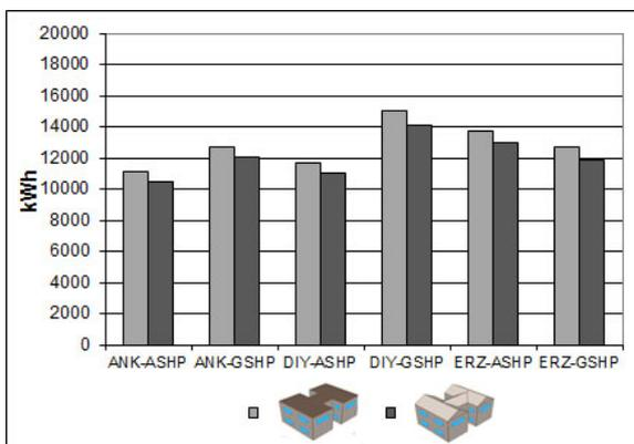
**Figure 7.** The comparison of annual energy consumption of flat and pitched roof when ASHP and GSHP systems are used in Ankara, Diyarbakir, Erzurum for H-shaped building form.
