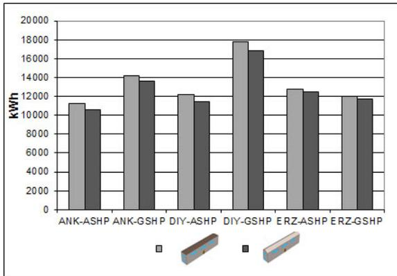
**Figure 5.** The comparison of annual energy consumption of flat and pitched roof when ASHP and GSHP systems are used in Ankara, Diyarbakir, Erzurum for rectangular building form.
