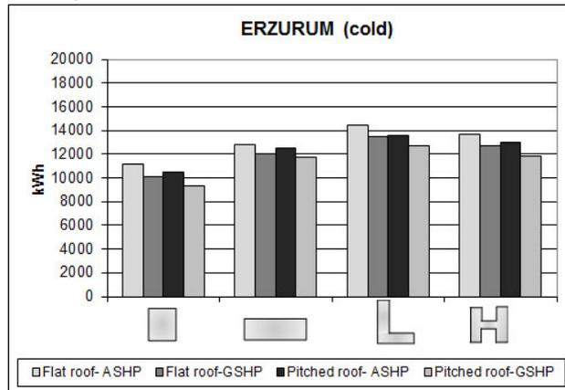
**Figure 3.** The comparison of annual energy consumptions of ASHP and GSHP systems in square, rectangular, L-shaped and H-shaped building forms for Erzurum.
