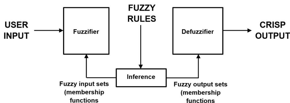
Figure 1. Conceptual scheme of a fuzzy logic system.
