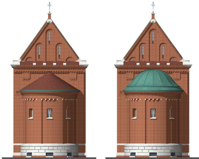
**Figure 7.** Conical (designed) and domed (built) form of the roof of the chapel apse. Reconstruction model (Source: Czechowicz).
