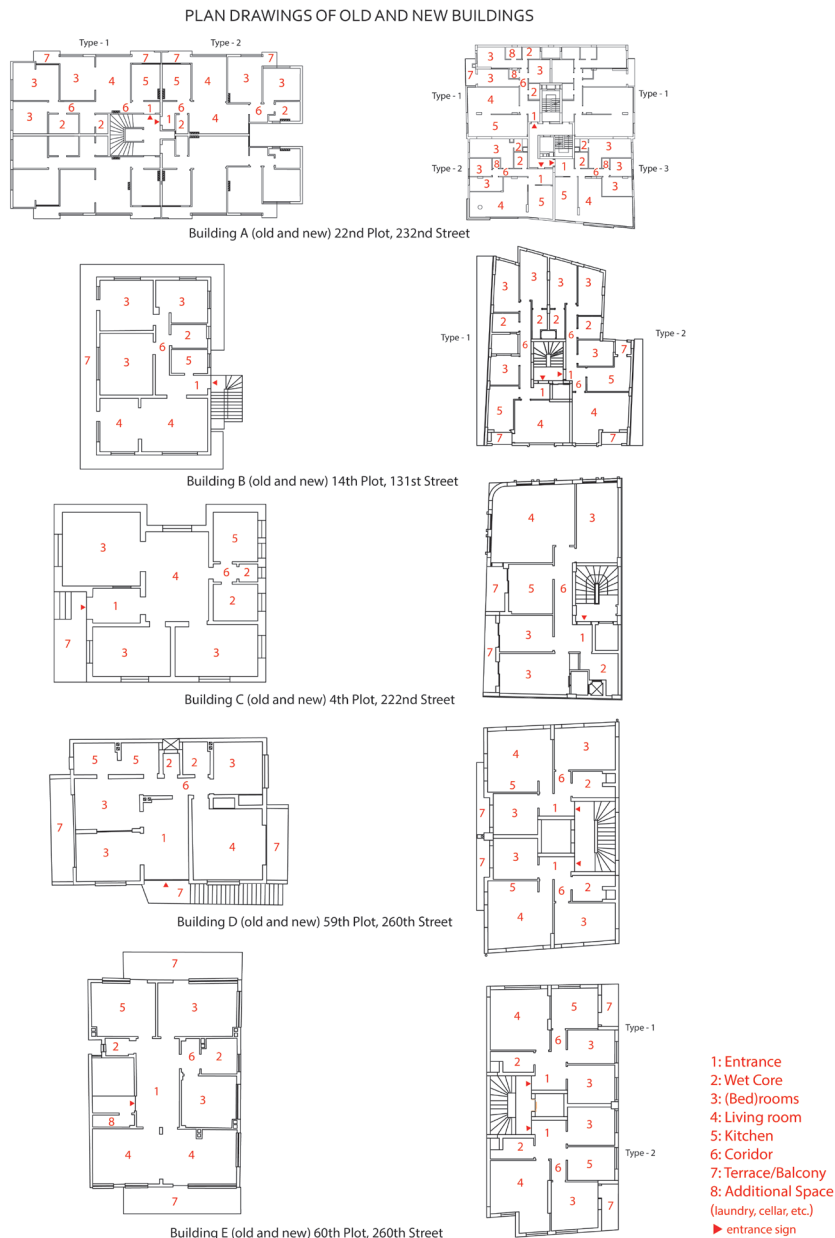
Figure 4. Plan drawings of the old and new buildings.
