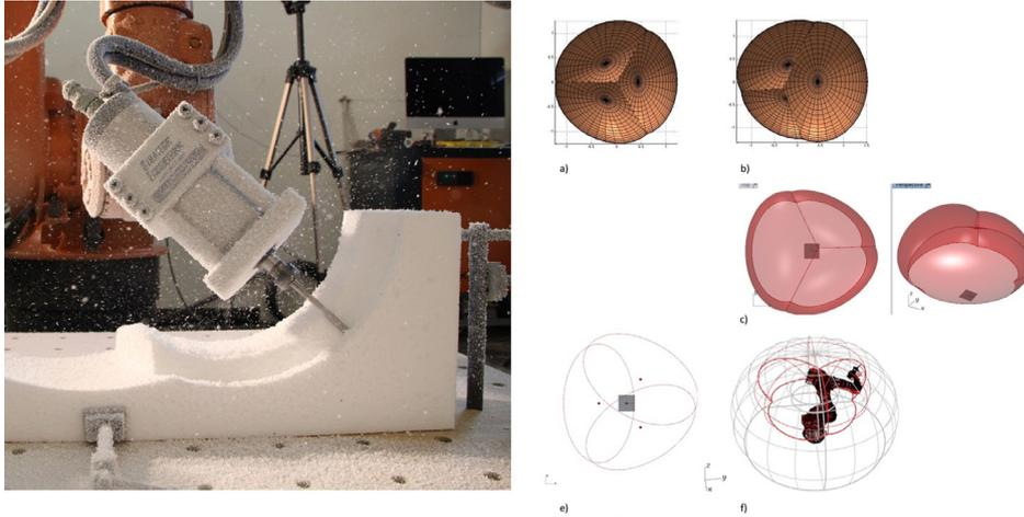
**Figure 6.** Shaping macro-geometries through robotic fabrication. Robotic acoustic prototype 1:4 scale model (left). Concept development (right): Generating Matlab function for primary geometry between homogenous 500-500-500 Hz space (a) and tuned ellipsoids as harmonic 400- 500-600Hz space (b) for ellipsoids; RhinoPython Code (c) and mapping producible space dimensions with constraints of robotic work envelope (f). Diagrams by author.
