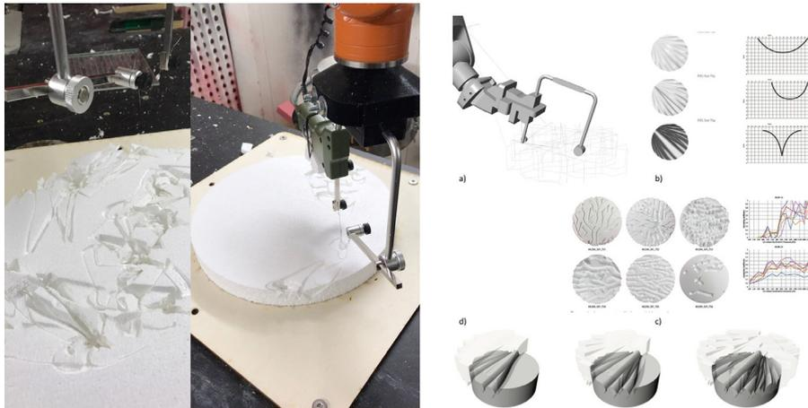
**Figure 8.** *Micropatterns as DNA of pattern script for robotic fabrication. Flocking based script for robotic fabrication (left). KUKA prc simulation with hotwire endeffector (a), sound discs relative to cutting profile changes (b) ; acoustic profiles for scattering and absorption performance (c), and reverse-engineering a mathematical relation between valley total, density and pattern depth. Images and diagrams by author.*
