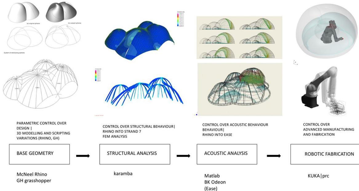
**Figure 9.** Workflow and range of variable parameter. Development of base geometries for spaces and intersections, principle testing of structural performance principle analysis of acoustic behavior of macro – and micro-geometries, application of robotic manufacturing protocols for modules or components, and surface patterns. Note that this is not a linear process, but recursive. Diagrams by author.
