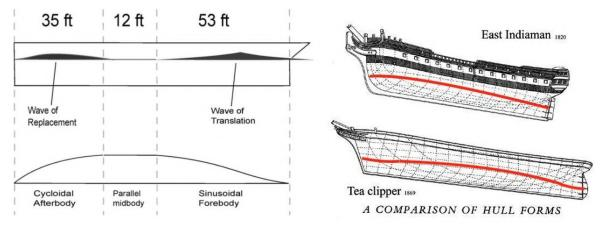
*Figure 3.* The wave generation of a hull, shaped according to the Wave-Line Theory (left top) and a half-top view of the waterline (left bottom) An East Indiaman Company Ship (right top), a Tea Clipper (right bottom). (Ferreiro and Pollara, 2016).
