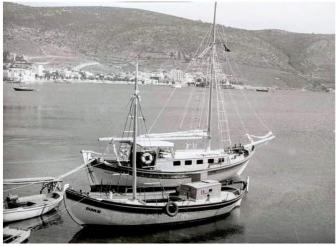
Figure 7. Two tirhandils, one open deck and one with cabin and pilot house (Sengün, 2017).
