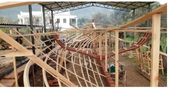
Figure 2. "Plank-on-Frame" technique (Kızılağaç, Bodrum, 2018).
