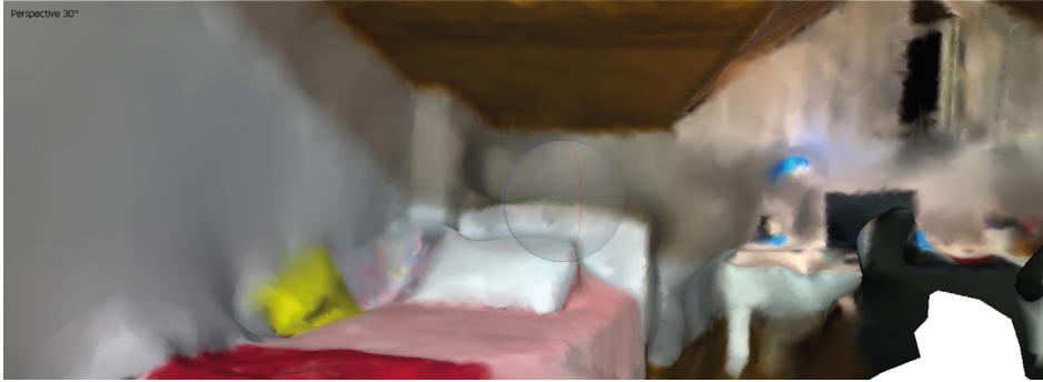
Figure 3. Model by S59 showing the consequences of skipping the 'building dense point cloud' phase.
