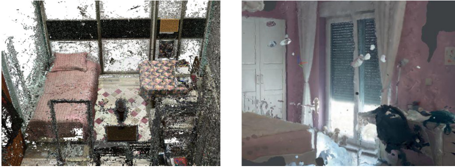
Figure 2. Model images of S56 with 570 photos (left) versus S53 with 75 photos (right).
