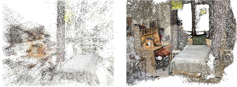
Figure 4. Images of the model by S36 that show the consequences of skipping the 'mesh building' phase.
