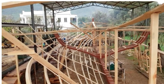
Figure 2. “Plank-on-Frame” technique (Kızılağaç, Bodrum, 2018).
