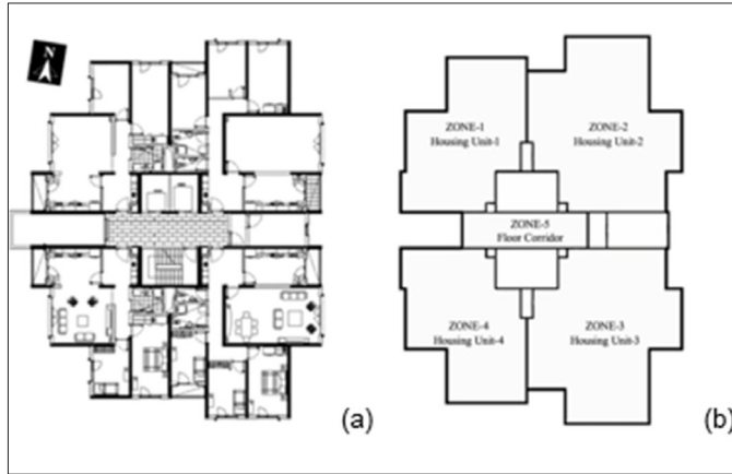
Figure 3. Plan view of the reference residential building (a) and conditioned zone areas (b).
