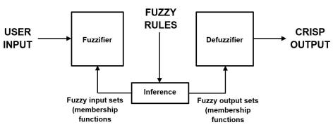
*Figure 1.* Conceptual scheme of a fuzzy logic system.
