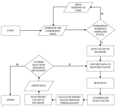
Figure 7. System evaluation algorithm.
