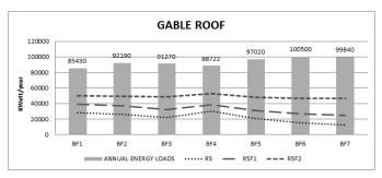
*Figure 4.* Annual energy loads and energy gains with photovoltaic systems in different building forms with gable roof.
