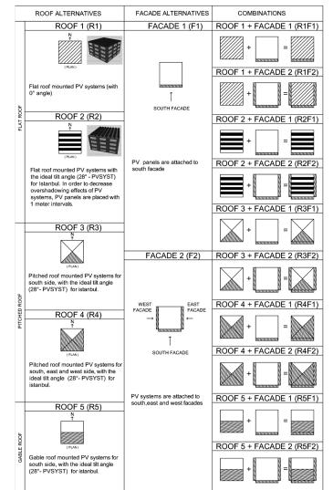
*Figure 1.* Roof and façade combinations for PV system installations.
