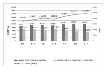
*Figure 6.* Annual energy loads, energy gains obtained with photovoltaic panels and lifecycle costs in different building forms for the R1F2 combination.
