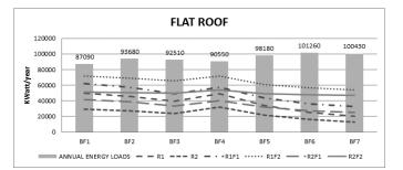
*Figure 2.* Annual energy loads and energy gains with photovoltaic systems in different building forms with flat roof.
