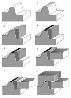
**Figure 1.** An animated demonstration of creating an "open" joint of external wall panels in a technological sequence.
