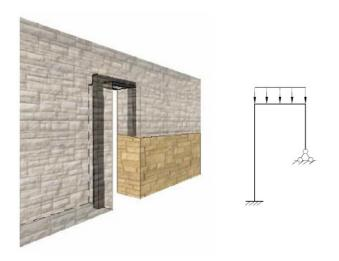
**Figure 6.** The scheme of calculation of a statically definable metal frame developed by a student on the example of reconstruction of a destroyed building wall.
