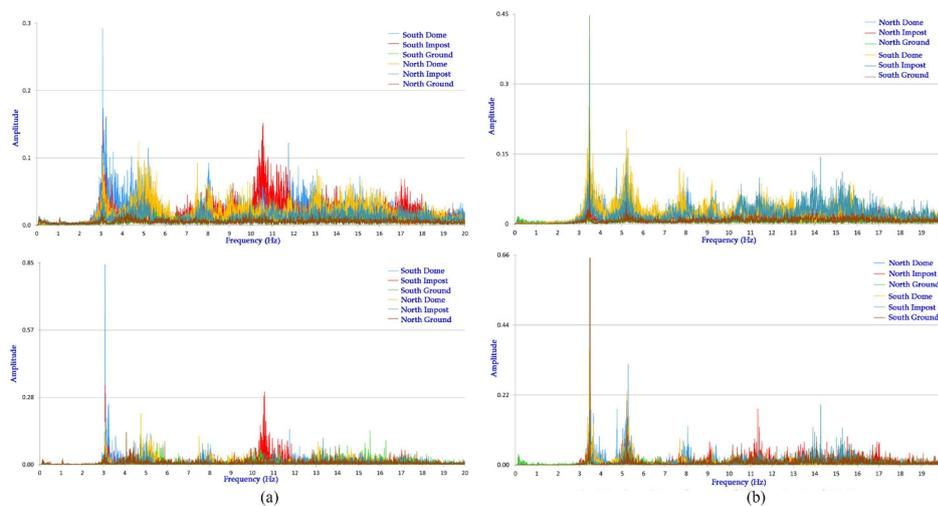
Figure 4. Fourier (above) and Power (below) Spectrums, a) Perpendicular to Qibla-x b) Qibla-y direction, (OMA-1).
