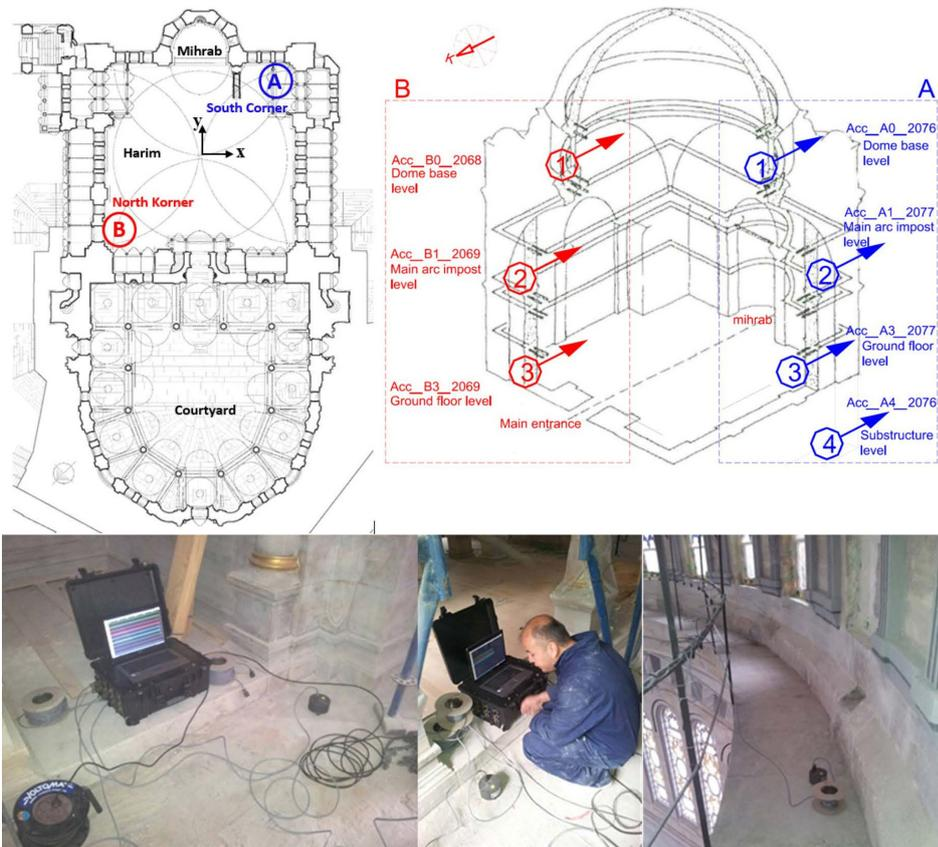
Figure 3. Setup for OMA-1 on plan and axonometric view, and data recording.
