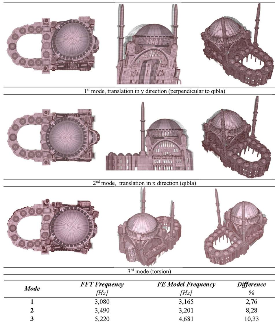
**Figure 8.** The first three mode shapes of calibrated FE model and comparison of experimental and numerical results.
