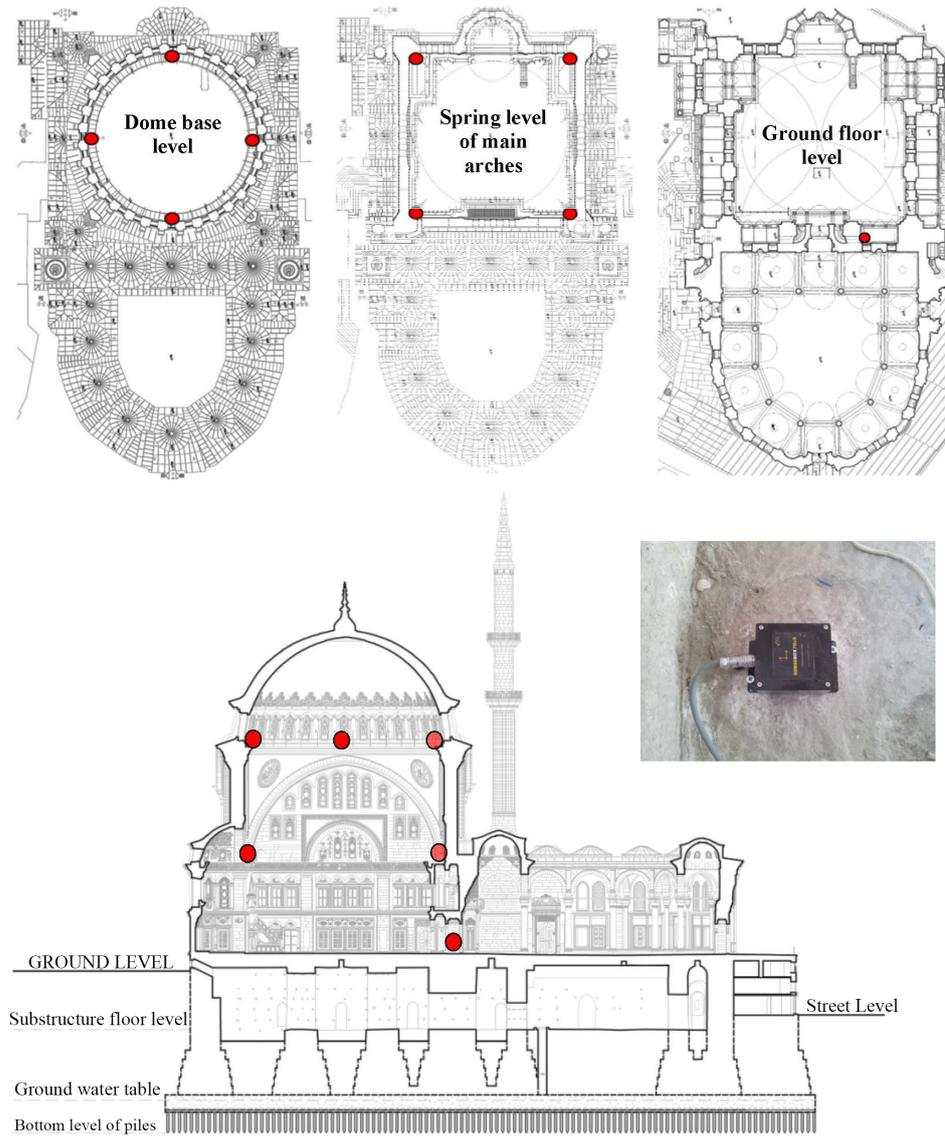
Figure 6. The locations of accelerometers on the plan and section of the mosque for OMA-2 test setup.
