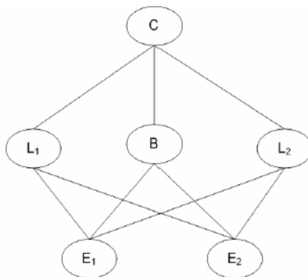
**Figure 5:** Control system syntax for the test bed ( $E_1$ ,  $E_2$ : illuminance sensors;  $B$ : device-controller for shades,  $L_1$  and  $L_2$ : device-controllers for Luminaires;  $C$ : Meta-controller)
