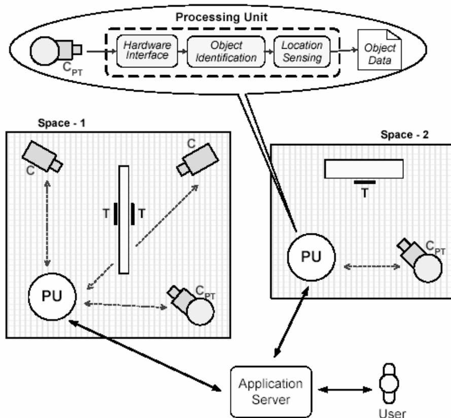
**Figure 8:** Schematic illustration of the overall structure of a location sensing system for sentient buildings (C: network camera; CPT network pan-tilt camera unit; T: optical tag; PU processing unit)
