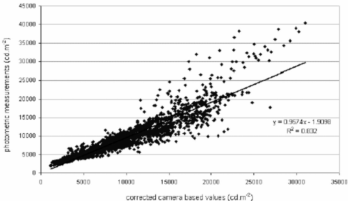
**Figure 7:** Photometrically obtained versus camera-based luminance values
