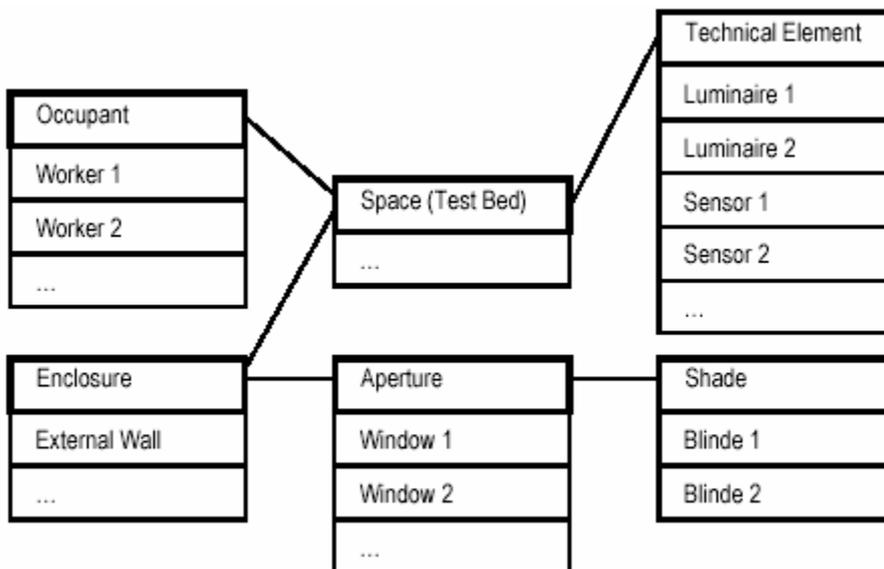
**Figure 4:** Product model scheme for the office space used as the implementation test bed
