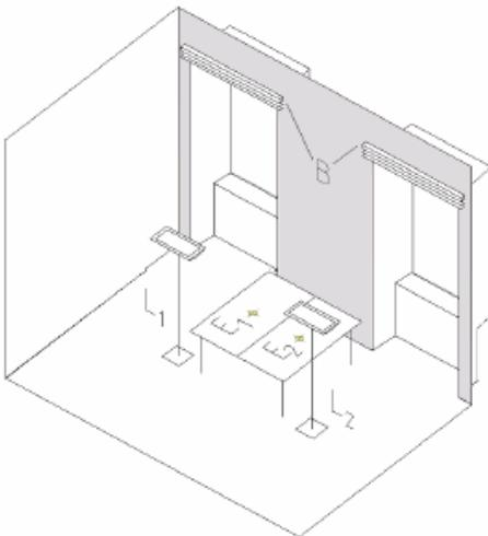
**Figure 2:** Schematic illustration of the office space (*B*: blinds;  $L_1$ ,  $L_2$ : luminaires;  $E_1$ ,  $E_2$ : illuminance sensors)
